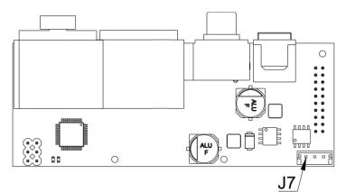
Figure 6: Dig-in IO pins, top view
