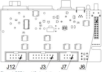
Figure 4: DSP board IO pins, bottom view
