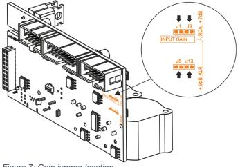
Figure 7: Gain jumper location
