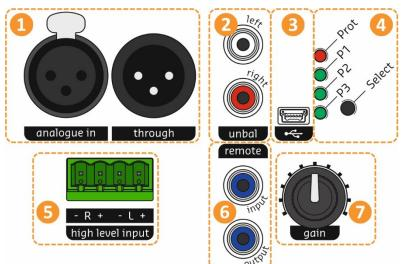
Figure 3: DSP with optional Sub input board
